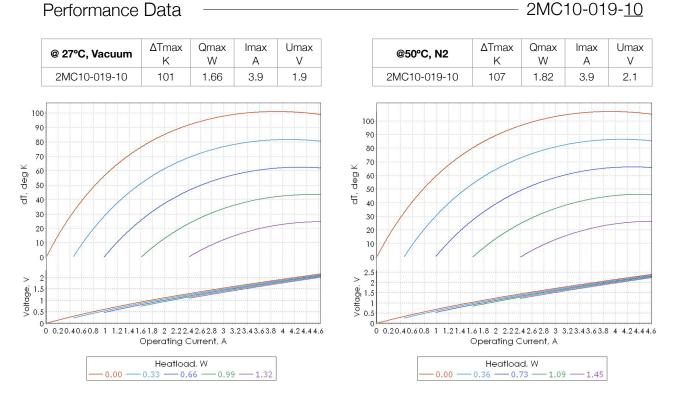
**Note**: Performance data is specified for optimal conditions (TEC hot side is stabilized at ambient temperature). Heatsink thermal resistance is not included into estimations. Use TECCad Software for estimations under different conditions.
